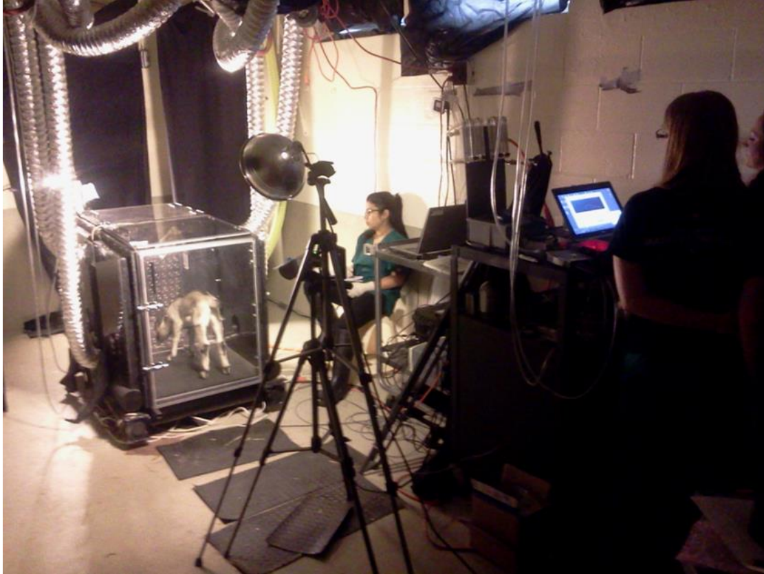
Figure 3.2 Test room setup showing kid in preference testing box, observer to right of test box, exhaust system, camera position, lighting placement and black curtains used for obscuring the observer from kid's view during preference testing of kids (n=12).
